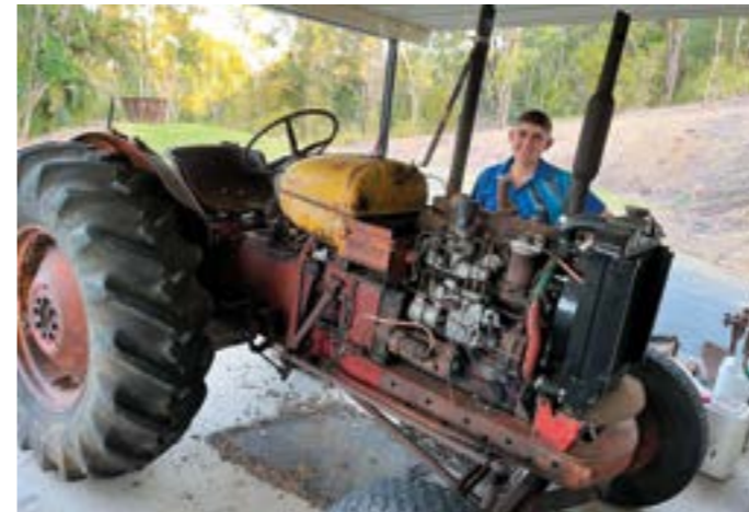
Restoration of this 1961-3 Nuffield 342 is an ongoing project for Travis and his Dad Chris. Work so far has focussed around the radiator, water pump and seals.
